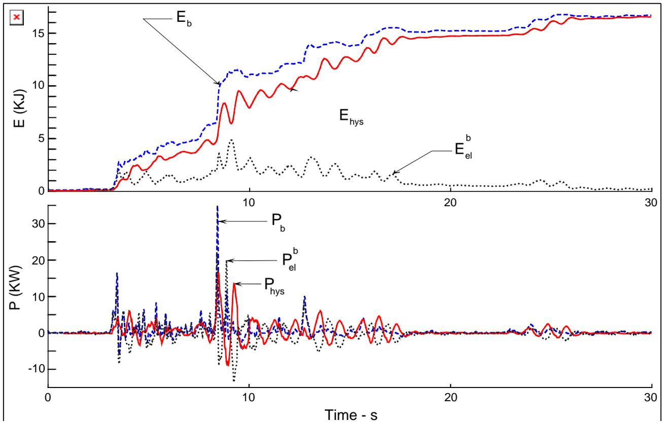
Fig. 8. Energy,  $E_b$  (top), and power,  $P_b$  (bottom), in the VN7SH building during Northridge earthquake, where  $E_{el}^b = E_b - E_{hys}$ .
