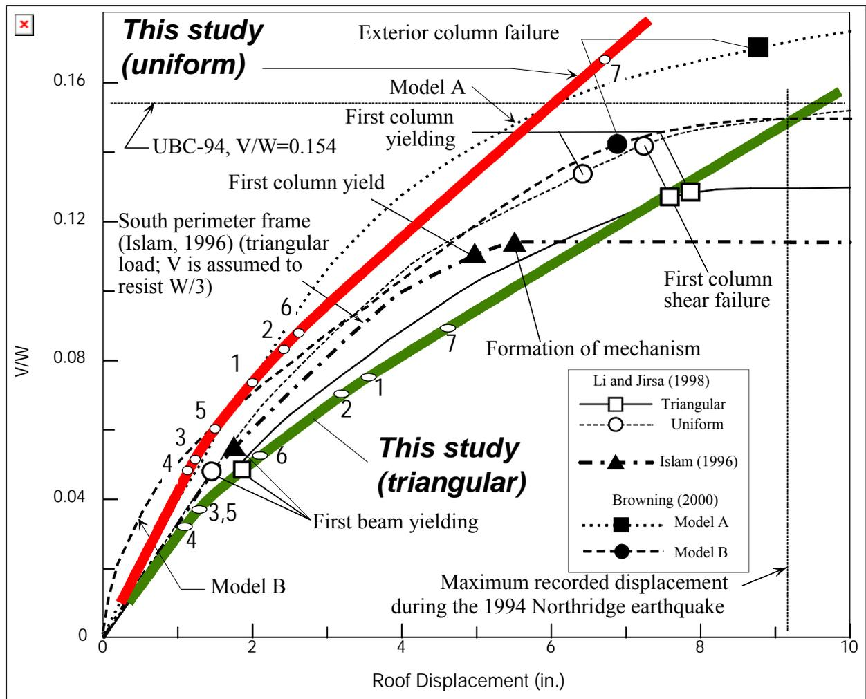
Fig. 4. Base shear ( $V$ ) coefficient normalized by total building weight,  $W$ , versus EW roof displacement of VN7SH (*This study* – open circles indicate first occurrence of nonlinear strain, at floors 1 through 7; Islam, 1996; Li and Jirsa, 1998; and Browning et al, 2000: Models A and B).
