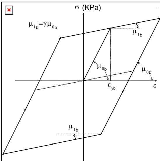
Fig. 7. Hysteresis loop representing  $\sigma(\epsilon)$  during time  $T_{0,i} < t < T_{0,i+1}$ .
