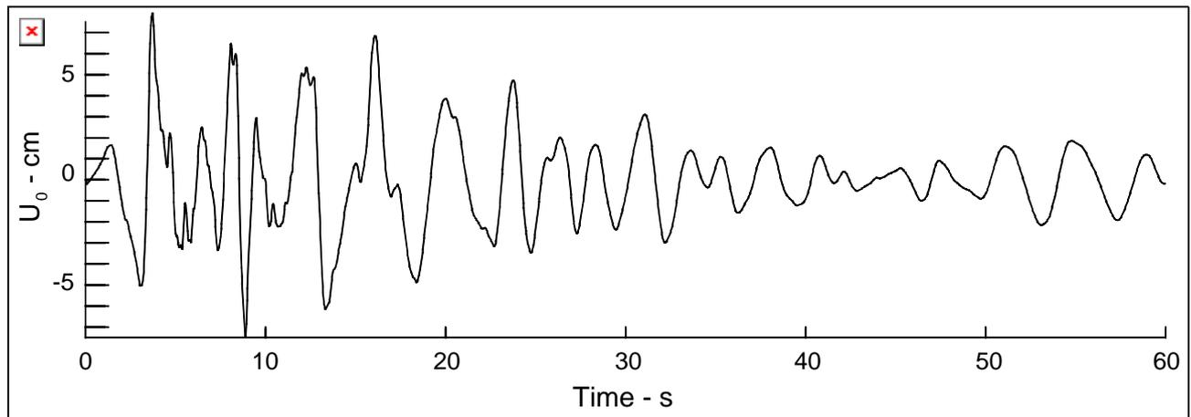
Fig. 5. Incident Ground Motion
