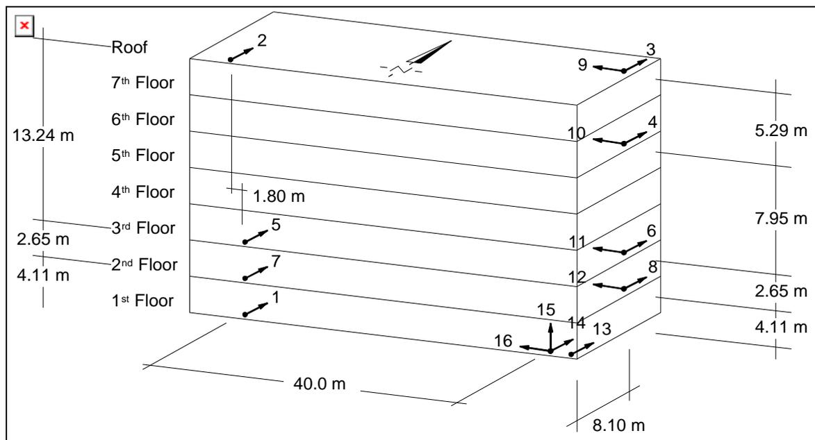
Fig. 3. Location of CR-1 channels (1-13), and of SMA-1 accelerograph (14-16).
