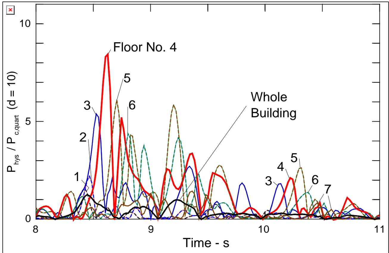
Fig. 12b. Normalized power demands in the model of VN7SH building, during excitation by Northridge earthquake, shown separately at seven floors, and in the whole building, for  $8 < t < 11$  s
