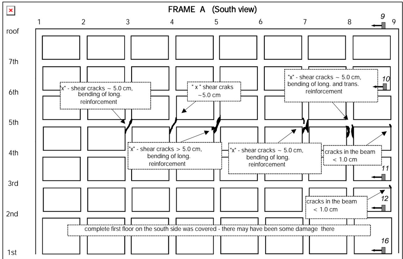
Fig. 2b. Observed Damage of Frame A.
