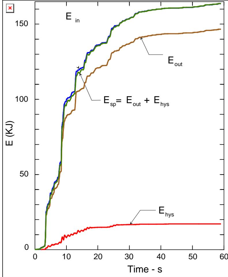
Fig. 6. Energy distribution in VN7SH, during the Northridge Earthquake. The spent energy consisting of energy going out of the building and the spent hysteretic energy, balance the input energy.
