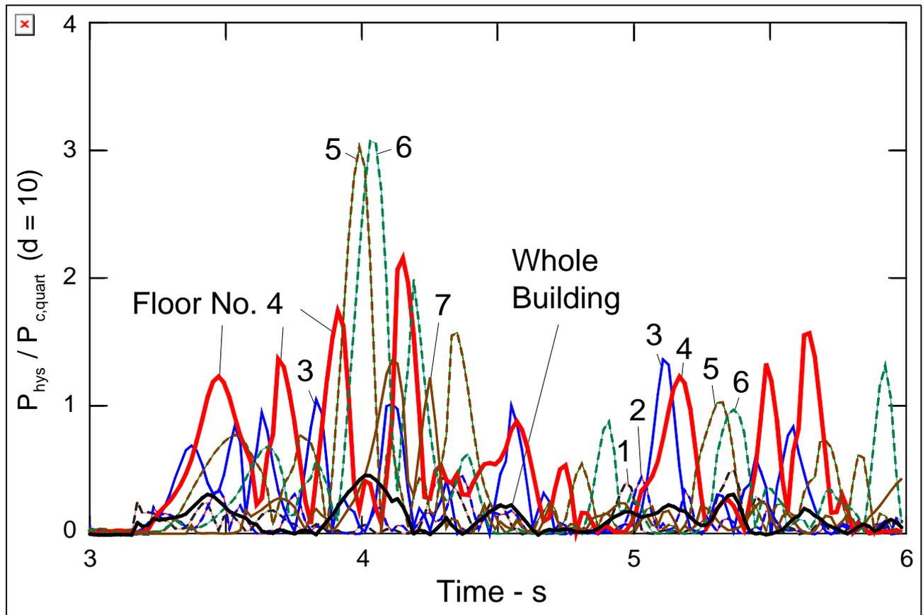
Fig. 12a. Normalized power demands in the model of VN7SH building, during excitation by Northridge earthquake, shown separately at seven floors, and in the whole building, for  $3 < t < 6$  s.
